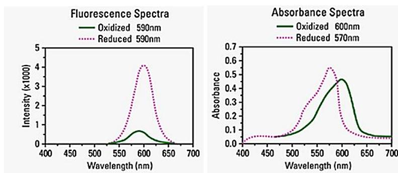
**Figure 2:** Fluorescence and Absorbance spectra of AlamarBlue Reagent in oxidized and reduced states
