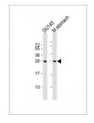
Lane 1: DU145 whole cell lysate Lane 2: mouse stomach lysate Lysates/proteins at 20 µg per lane. Secondary Goat Anti-mouse IgG, (H+L), Peroxidase conjugated at 1/10000 dilution. Predicted band size : 25 kDa Blocking/Dilution buffer: 5% NFDM/TBST.
